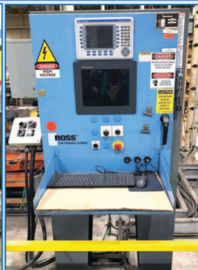
ROSS INDUCTOHEAT FLUXMANAGER PIPE END STRESS RELIEVING SYSTEM
